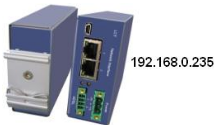
Figure 3.43: The default IP address for a DINrail unit is 192.168.0.235.
