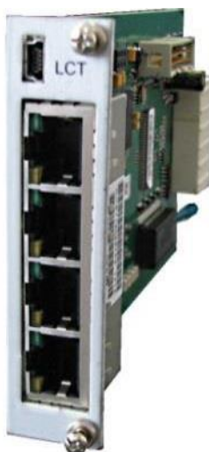
Figure 3.33 Managed Switch Line Card
