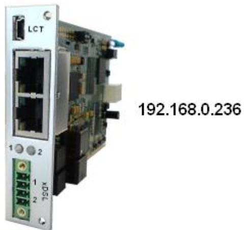
Figure 3.47: The default IP address for a single delivered line card is 192.168.0.236.
