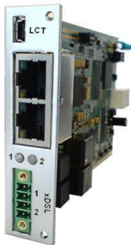
Figure 3.16 SHDSL Line Card
